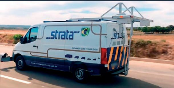
**LASER CRACK MEASUREMENT SYSTEM**
